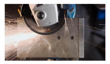
Hit the mark with pinpoint precision: the disc becomes transparent when it rotates, enabling precise working
